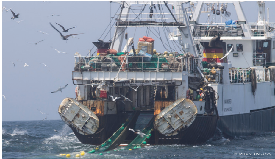
A midwater trawler retracting gear through the stern ramp
