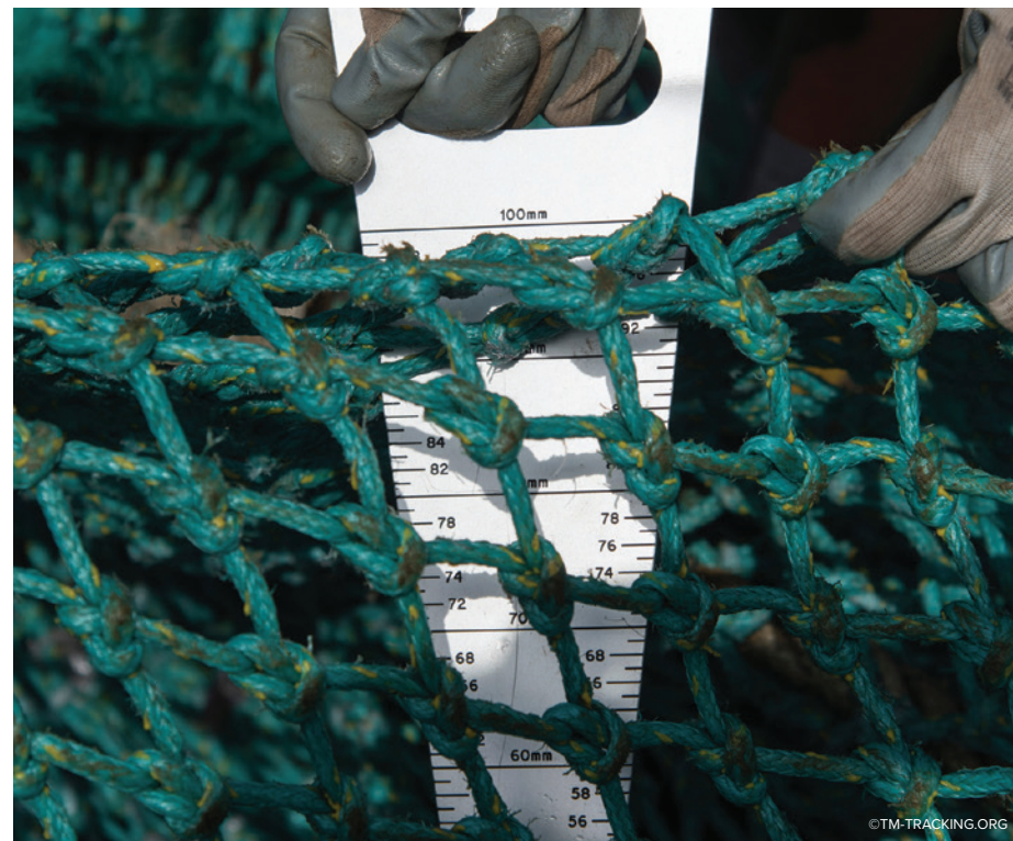
The size of the mesh can be measured using a specialised tool called a net gauge
