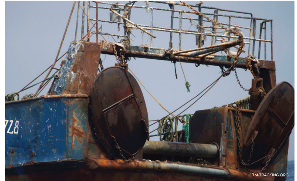
A trawler with the trawl doors stored
