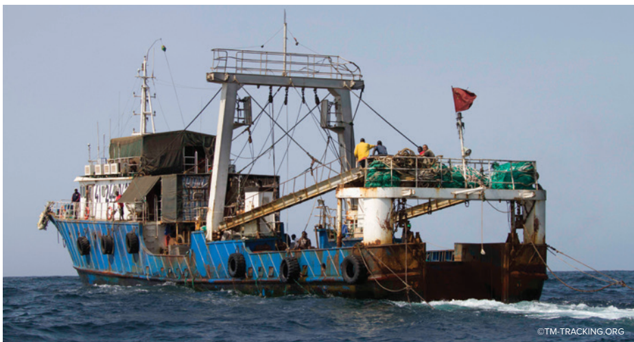
A trawler with warps in the water, indicating that it is actively fishing
