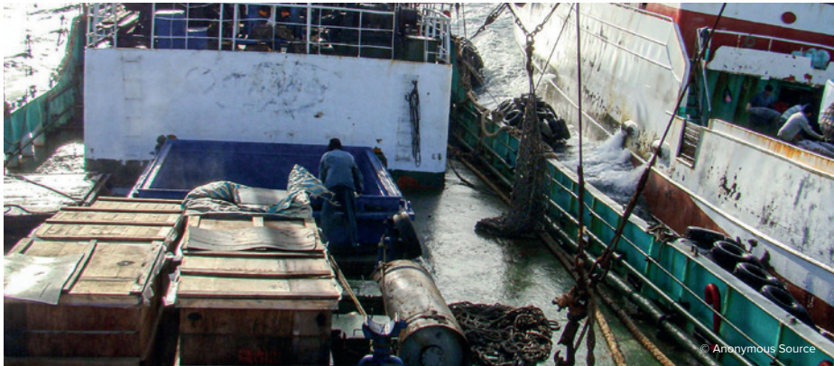
(Above) Longline vessel transhipping to a carrier vessel at sea. The use of large Yokohama fenders can be observed.
