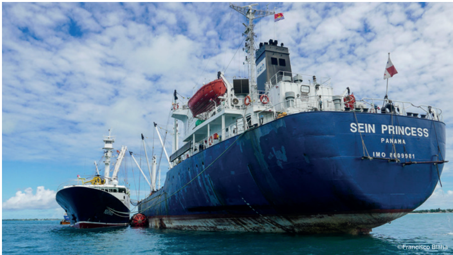
Transshipping at anchor in port area. Note the large 'Yokohama' fender deployed between the carrier and unloading vessel.
