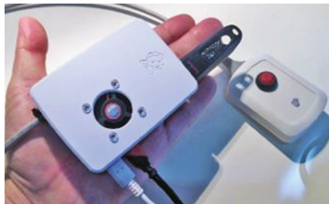
Data logger is built from a Raspberry Pi microcomputer and Actisense NDC-5 Multiplexer.
