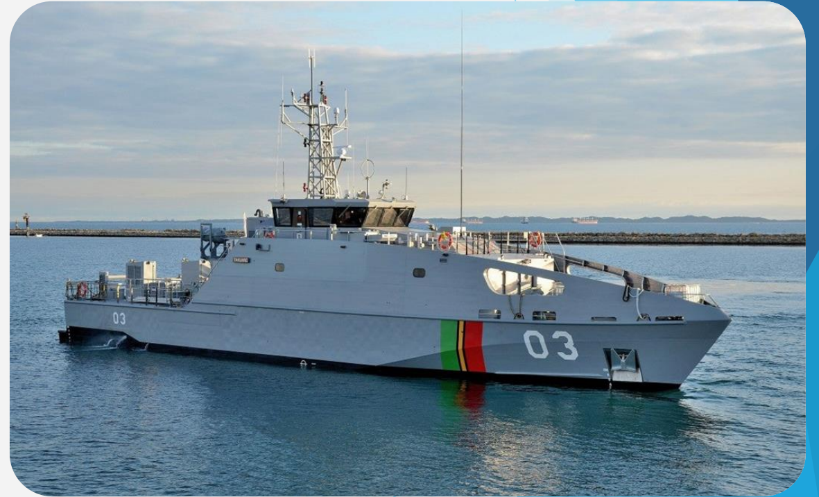
RVS Takuare is a 39.5m steel monohull Guardian-class Patrol Boat
