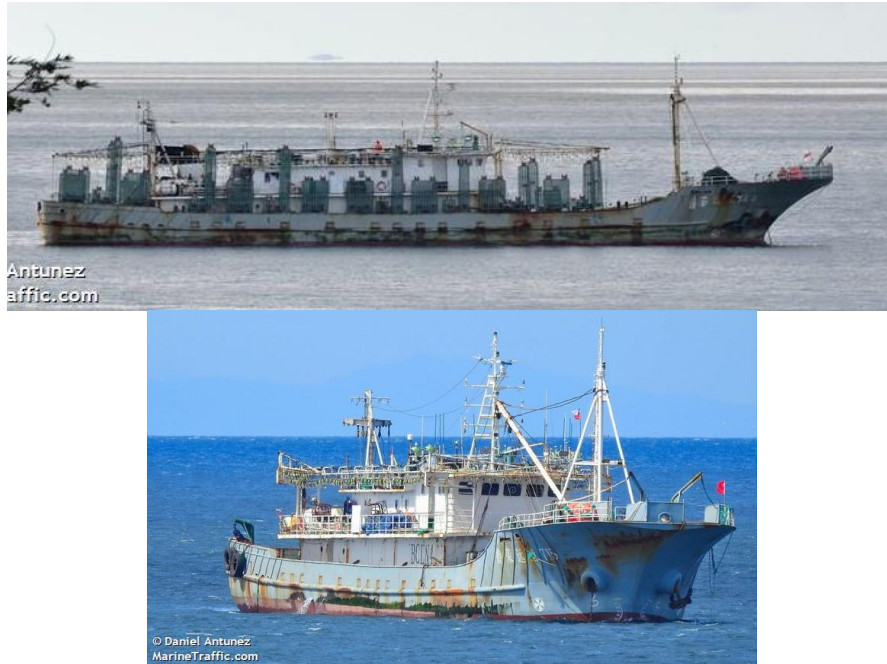
Figure 12 - LU RONG YUAN YU 715 observed in Punta Arenas, Chile in June 2020 (top) configured for squid jigging and configured for trawling in November 2021 (bottom) 38 .
